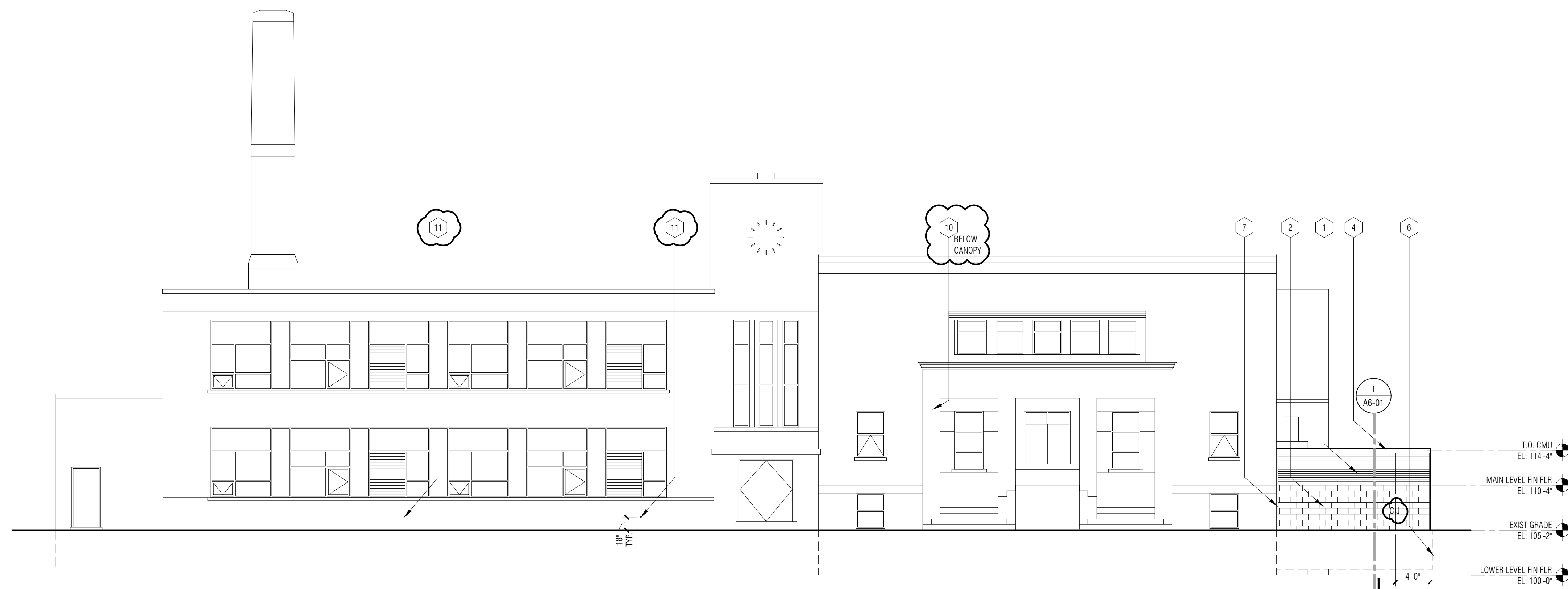
1 West Exterior Elevation A3-01 1/8" = 1'-0"
